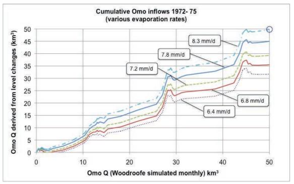
Figure 87: The Omo's cumulative "modelled" & "simulated" runoff, 1972-75, for various evaporation rates
