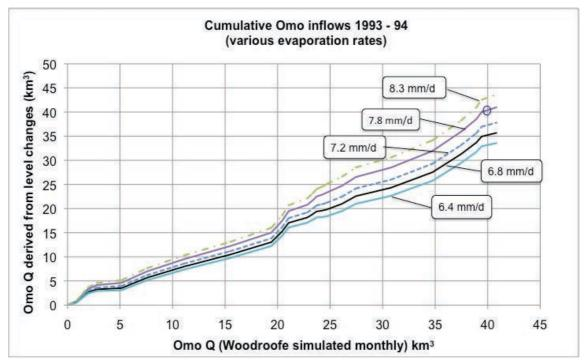
Figure 88: The Omo's cumulative "modelled" & "simulated" runoff, 1993-94, for various evaporation rates
