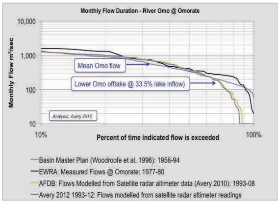
**Figure 94: Flow duration curves for the Omo River at Omorate** *Data Sources are indicated in the above graph's Legend.*
