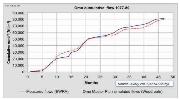
Figure 46: Omo River simulated & measured runoff compared from 1977 - 1980
