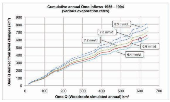
Figure 86: The Omo's cumulative "modelled" & "simulated" runoff, 1956-94, for various evaporation rates
