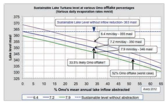
Figure 98: Lake drawdown – Sensitivity of modelled lake level to three different assumed evaporation rates
