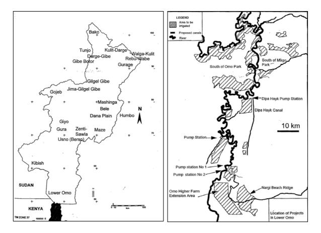
**Figure 8: Potential irrigation areas studied by the Omo-Gibe Basin Master Plan** *Graph on LHS. Source: Woodroofe, Vol. XI, F2, Figure A1, p41.*
