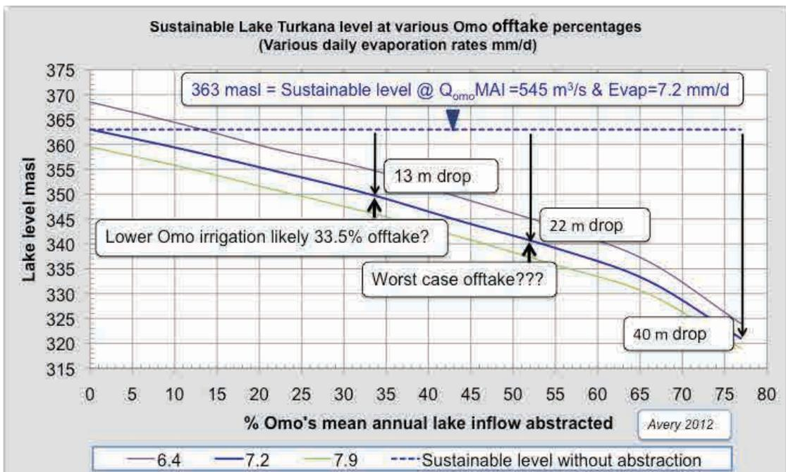
Figure 99: Lake equilibrium level reduction with increased Omo offtake (at 7.2 mm/d evaporation)
