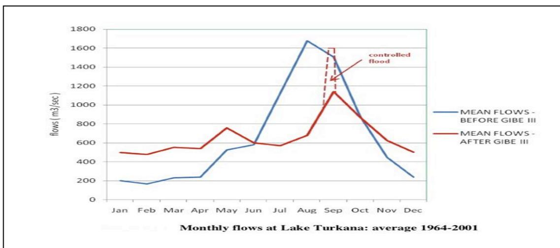
**Figure 4: Proposed regulated flow sequence from the Gibe III hydropower project**
