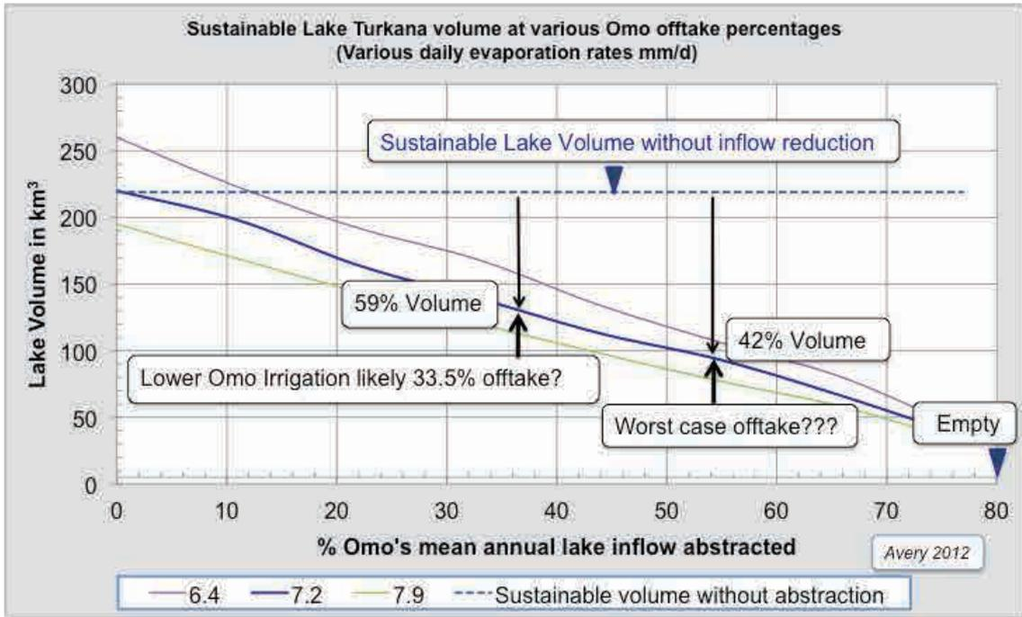
**Figure 100: Lake equilibrium volume reduction with increasing Omo offtake (at 7.2 mm/d evaporation)**
